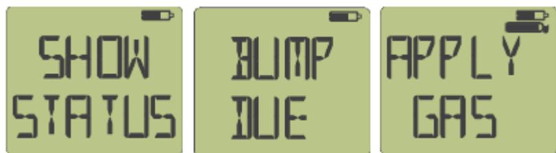
The detector will flash between "BUMP DUE" and "APPLY GAS". Apply gas to the unit at a flow rate of 0.25 to 0.5LPM using the calibration cap provided. Once all sensors have gone into alarm, the unit will return to normal operation (in alarm) and the bump due date will be reset.
